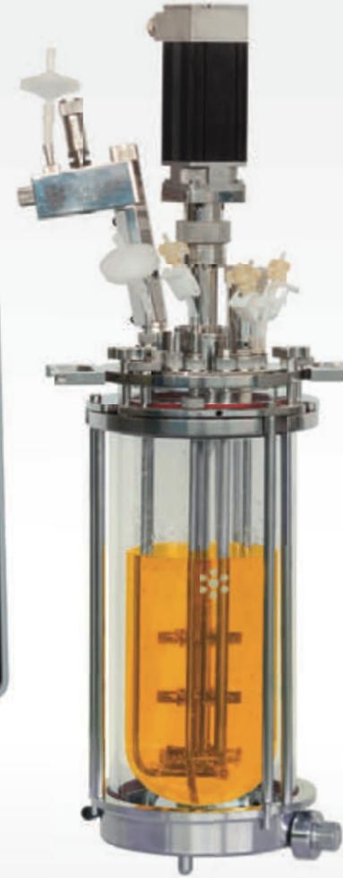
Powerful/ Accurate **brushless motor**, from 1 to 2000 RPM.
