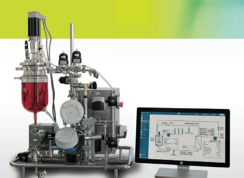
KRONOS is a standalone, benchtop, automatic Tangential Flow Filtration (TFF) system offering up to 0.5 m2 total filtration area. Utilizing state of the art componentry, the system is equipped with powerful software enabling automatic process sequences, and innovative process development modules.
