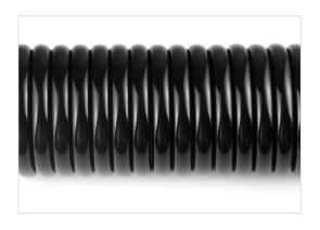
Envir-A-Line XX is commonly used for many **gases** and **hydrocarbons**. has a unique **coextruded** construction, incorporating a highly inert Hytrel™ inner-liner that exhibits excellent dielectric properties and provides a superior **gas** and **moisture barrier**. Its moisture permeability is similar to poly-ether based urethanes. The product's outer shell is comprised of a permeable photo-opaque black PVC, so the product can be repeatedly autoclaved without the two materials separating.
