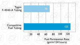
The performance of tubing is affected by the conditions of use and equipment utilized, along with size and wall thickness of the tubing tested. The data above is presented for information only and should not be utilized for specification purposes.
