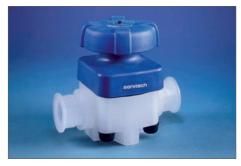
For use in high-purity water, chemical and process lines. Valves have a smooth fluid path with no pockets to harbor bacteria or contaminants. Fluid comes in contact with only two valve components, the body and diaphragm. These valves can be pneumatically actuated.
